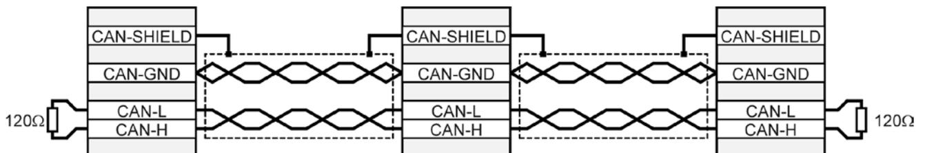
Figure 22: Cabling example for CAN-Bus
