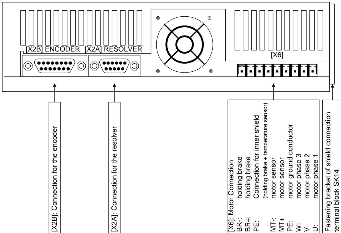
Figure 13: item servo positioning controller C 1-02: Bottom view
