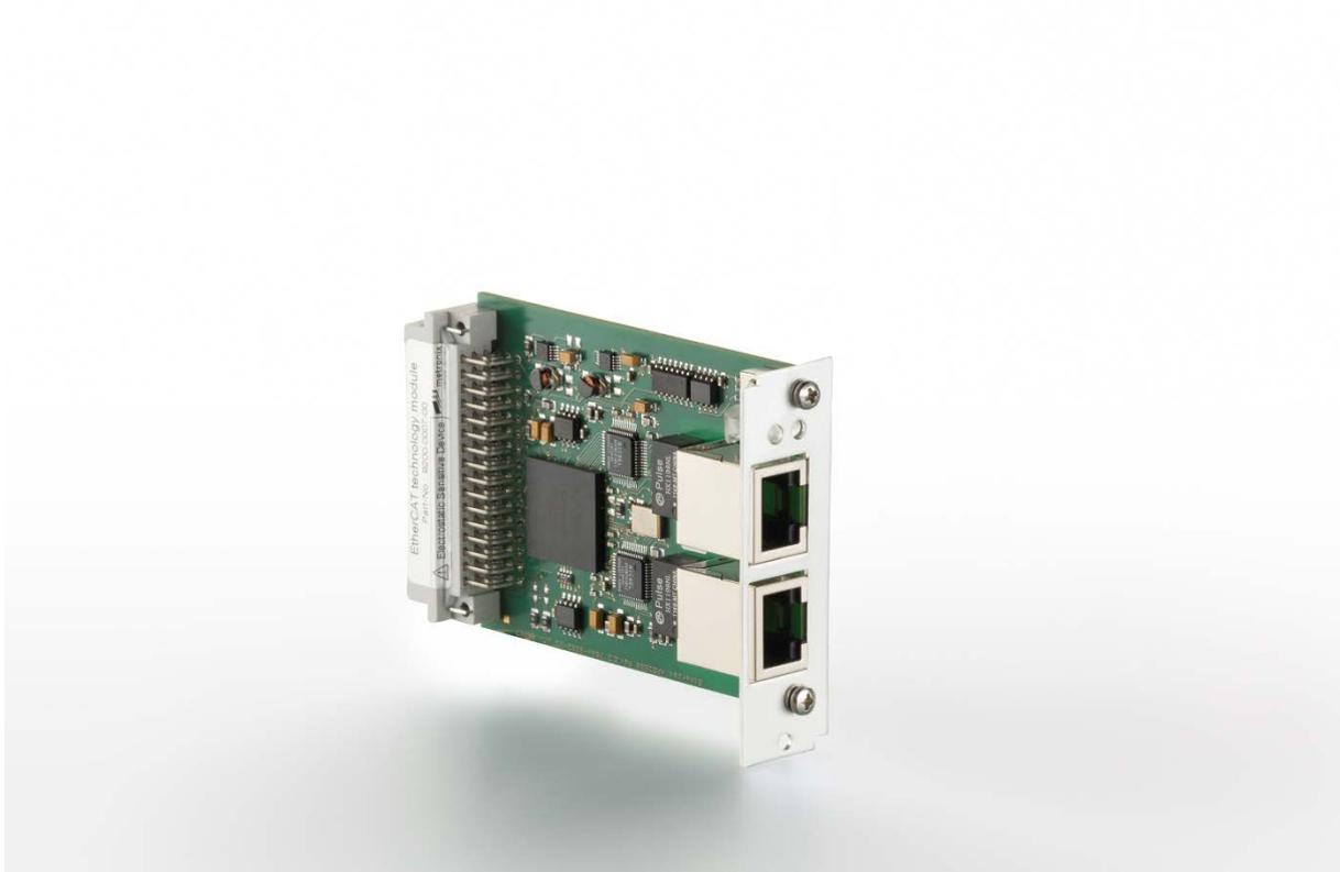
Figure 29: EtherCAT module: Front view
