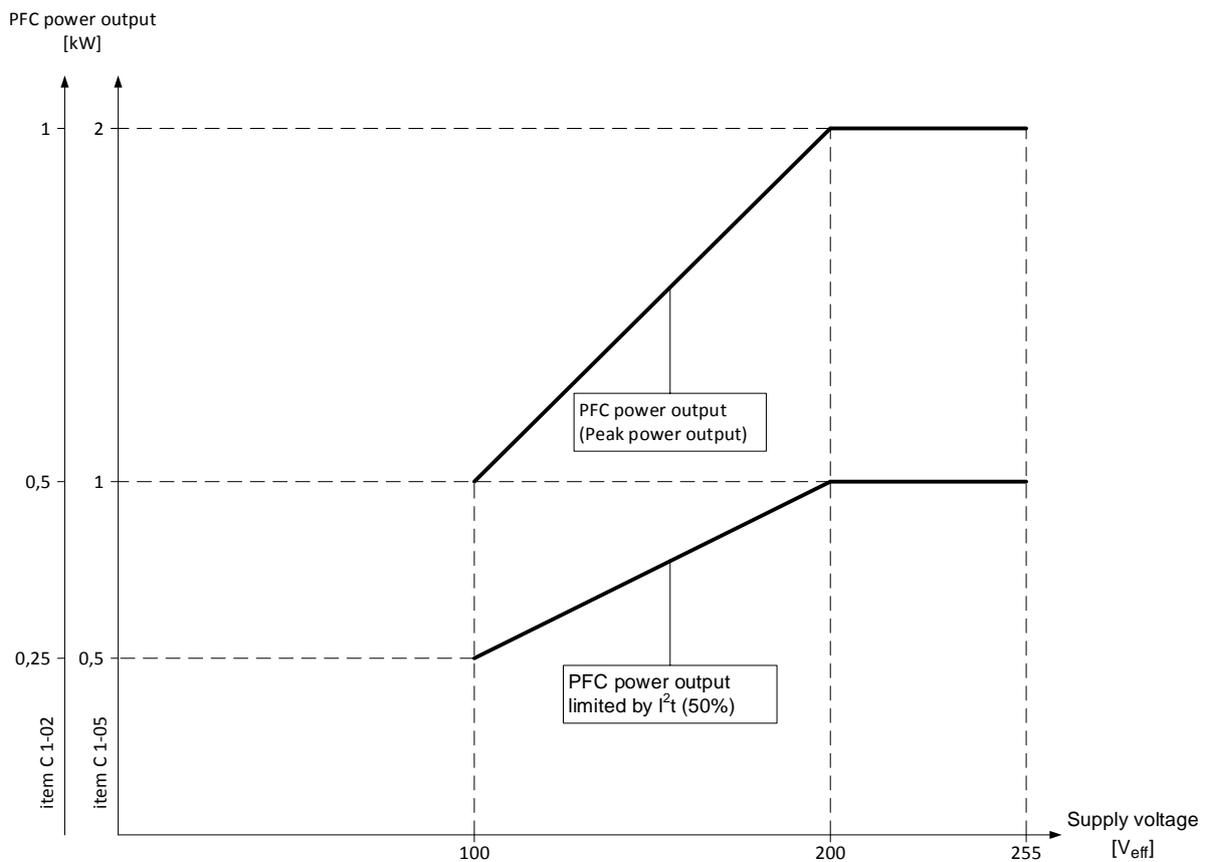
Figure 3: Performance curve of the PFC stage
