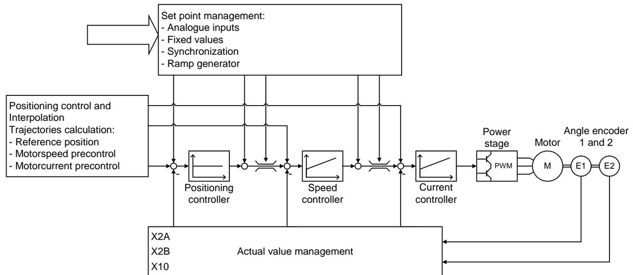
Figure 4: Control scheme of the item C 1-Series
