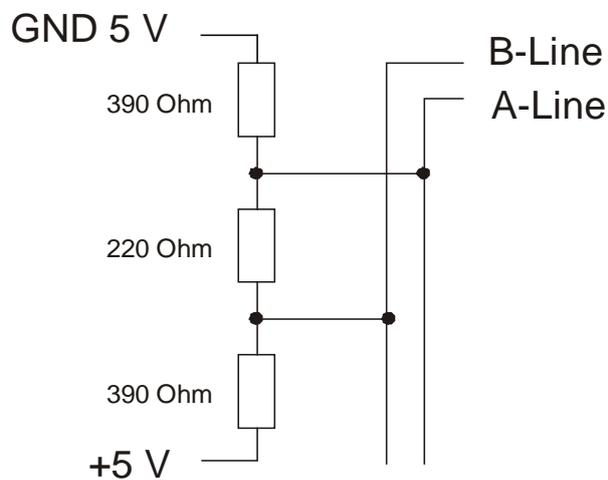
Figure 28: PROFIBUS-DP interface: Connection with external terminating resistors
