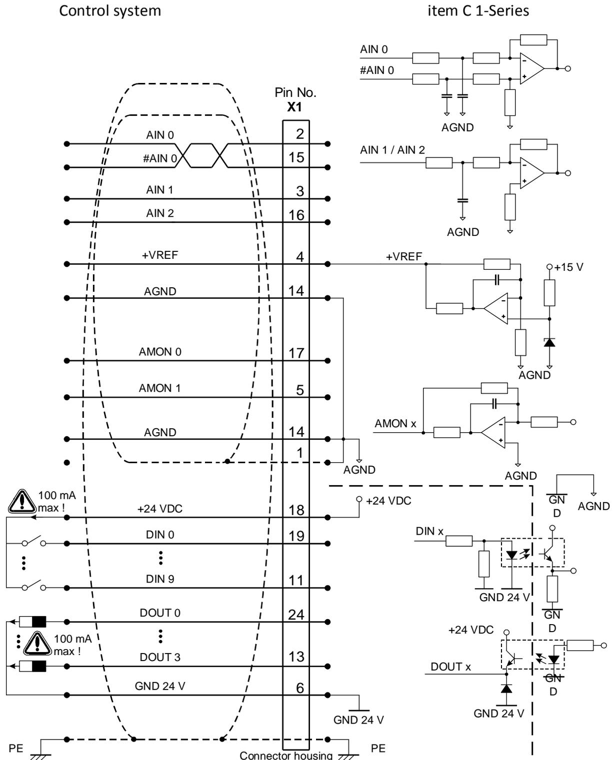
Figure 20: Basic circuit diagram connector [X1]
