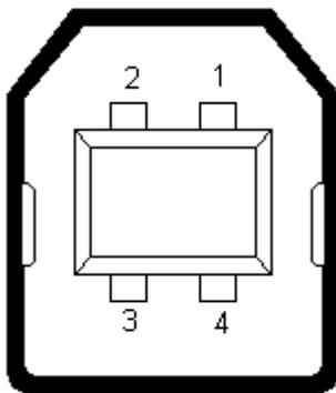
Figure 25: Pin assignment: USB interface [X19], front view
