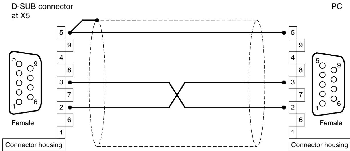
Figure 24: Pin assignment: RS232 null modem cable [X5]
