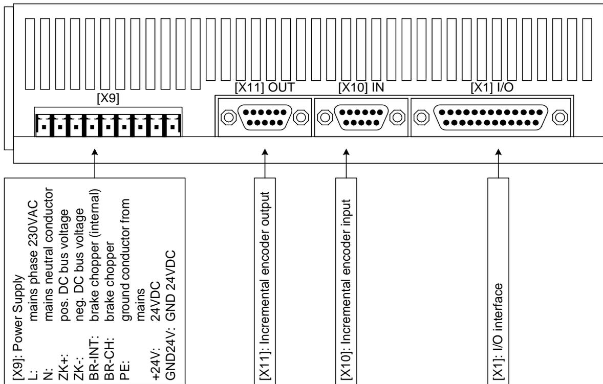
Figure 12: item servo positioning controller C 1-02: Top view
