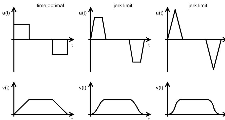
Figure 5: Driving profiles of item servo positioning controller C 1-Series
