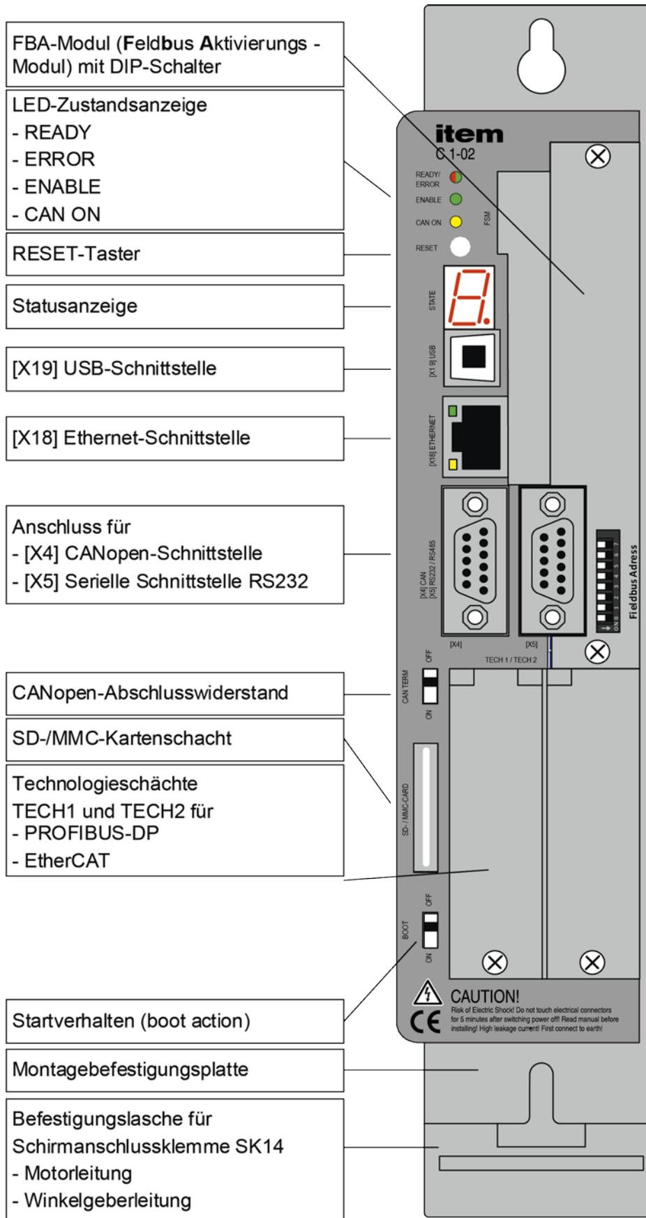
Figure 11: item servo positioning controller C 1-02: Front view
